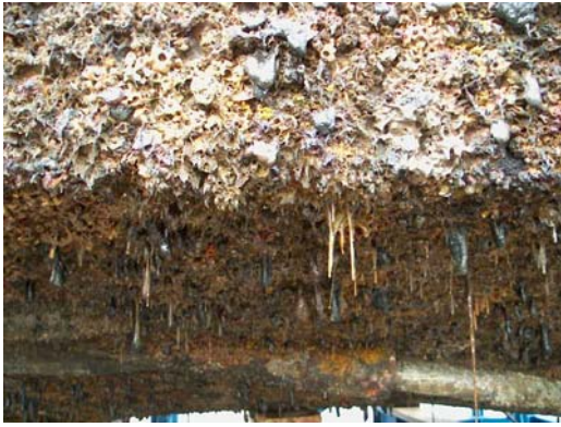
Figure 5. When the antifouling paint is not effective anymore, a ship can become as severely fouled as shown in the picture. With this amount of attached biological material, the ship is neither safe nor suitable for transportation. (With permission, Johnny Eliasson, Stolt-Nielsen, NL).
