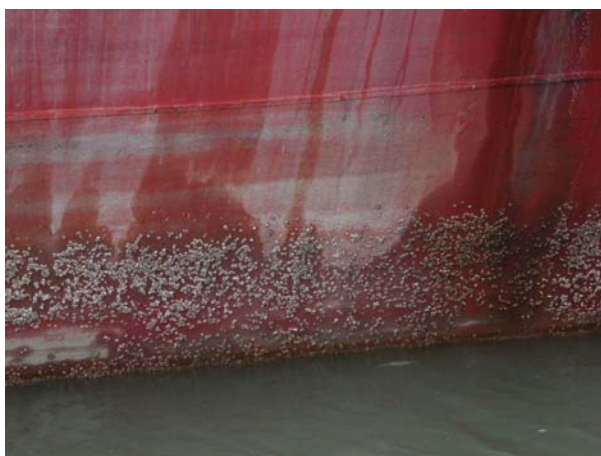
Figure 8. A ship's hull with barnacles. When a ship looks like this, it is too slow and consumes too much fuel. The ship will become too expensive to use for transportation and at the same time, increases the emission of green house gases. (With permission, Johnny Eliasson, Stolt-Nielsen, NL)
